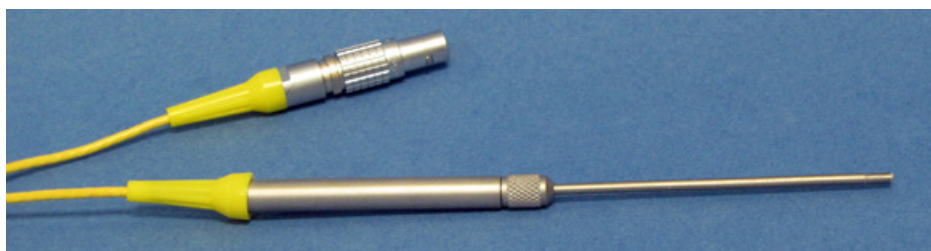
Fig. 1—The ISO-HPO-2 sensor works with WPI free radical analyzers to monitor hydrogen peroxide.
